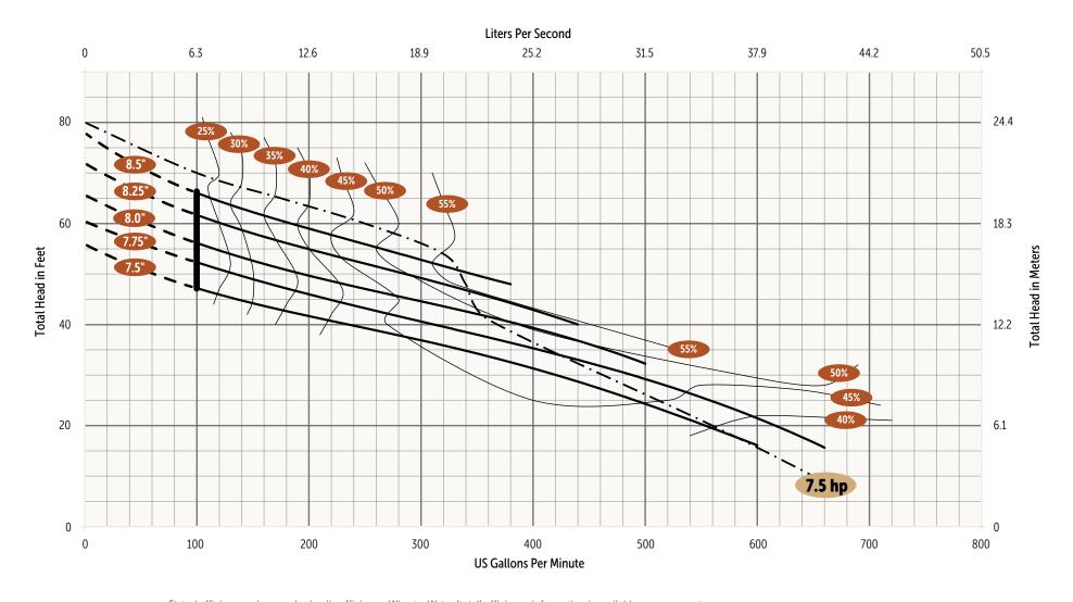
Stated efficiency values are hydraulic efficiency. Wire-to-Water (total) efficiency information is available upon request.
